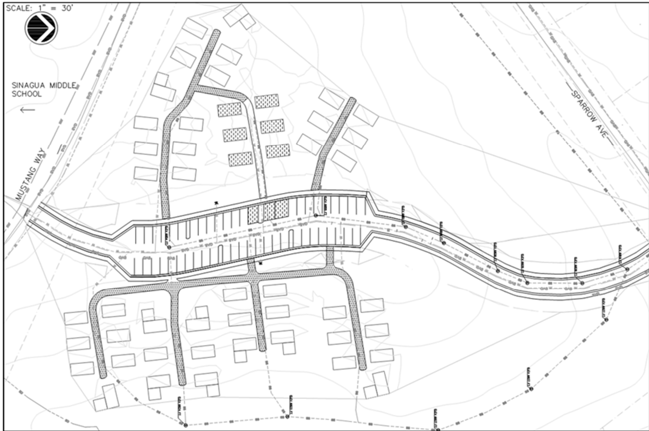
Figure 5: Utility Layout for Tiny Home Site Design Showing Sewer Line Connections Back to Proposed Road
